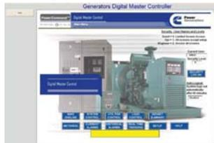
The PLC at the 3.3kV Substation provides control and monitoring of the 3.3kV Distribution. The area of the 3.3kV Substation also includes interfaces to substation protection relays and the Digital Master Controller (DMC) for the Standby Generators.
